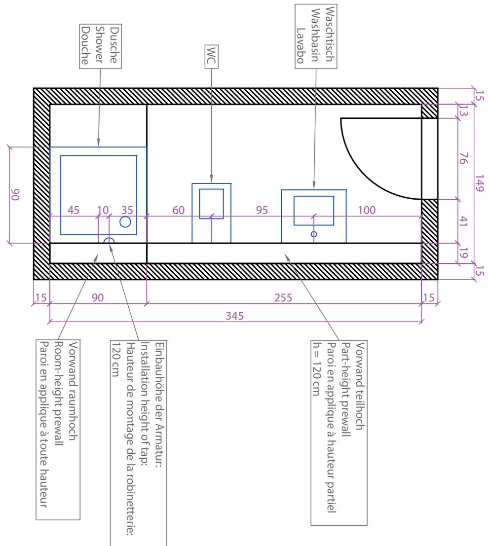
Fig. 6-1 Small bathroom planning example (all dimensions in cm)
