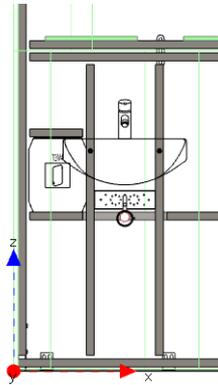
7. In the **Masonry walls and installation walls** window, select **Mounting plate**.
