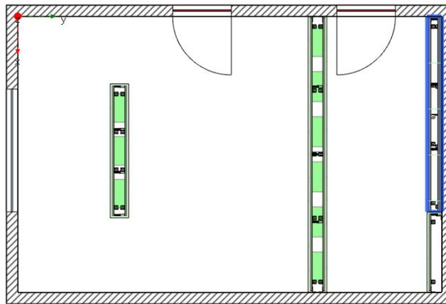
**Inserting the second room-height prewall**
